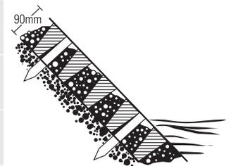
\*A slope of 1 in 1 is possible if every block has suitable anchoring in one of the cores into the subsoil and the site has been assessed to ensure global stability is not an issue.
